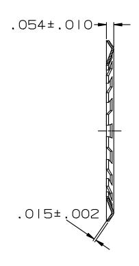
MATERIAL: SAE 1060-1090 SHAFT DIA: .995-1.005 (1") (25.4mm) NOTE: 18 TEETH EQUALLY SPACED
