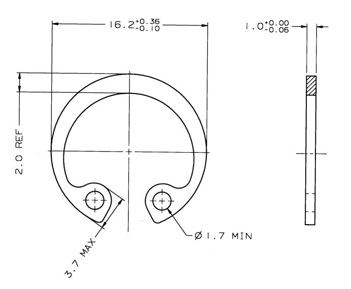
HOUSING DIA = 15.0 GROOVE DIA = 15.7 GROOVE WIDTH = 1.10 MIN MATERIAL: SAE 1060-1090 HARDNESS: 470-580 HV (47-54 HRC EQUIV.)
