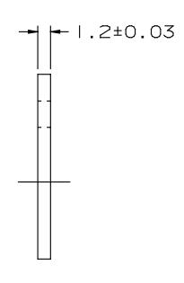
SHAFT DIA: ||.0 - |5.0 GROOVE DIA: |0.0 %: % GROOVE WIDTH: |.25 %: % HARDNESS: Rc 46-54
